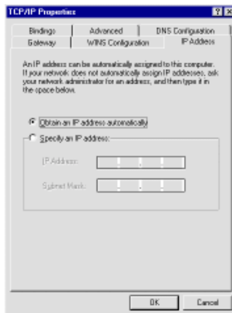
FIGURE 8: TCP/IP Properties screen with Obtain an IP address automatically selected
